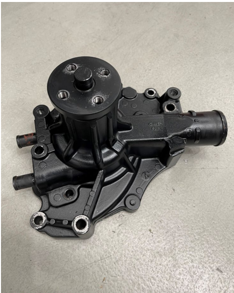
10PK HD Drive Early Style Water Pump (GMB) - SBF 5.7" tall, 5/8" pilot, Driver Inlet (Use with Early Model Mechanical Fuel Pump Timing Cover, or Dorman 635-107)
